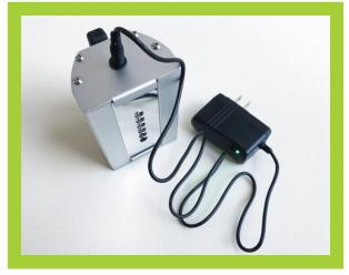
When charge, the light shows the charge status of the device. Red means charging; Green means full charged.
